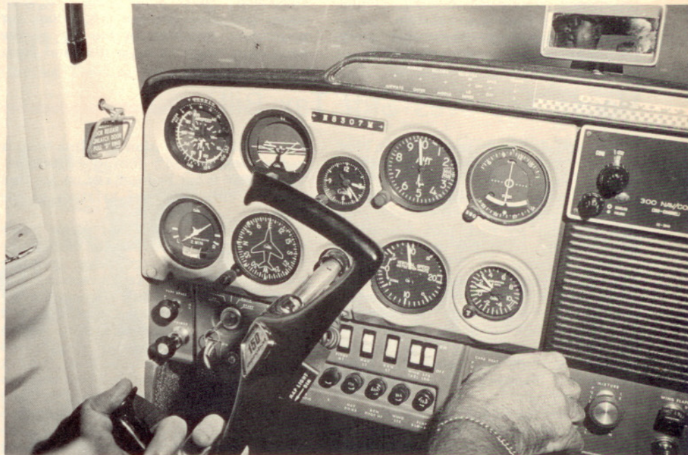
Barrel roll at the inverted point. Note gyro-horizon, aileron deflection, and plus one-quarter G force. IAS is 108 m.p.h., and the aircraft is still going up.
