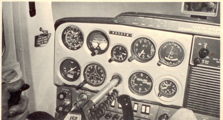
This photo was taken by Chuck Hinson as author Downie "fell out of the top" of a too-big loop. Airspeed is almost zero; rate of climb over 2,000 f.p.m. (There is a lag in indicator.) Plane had just been kicked off to the left to avoid a tailslide.
